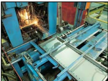
Automated welding of Hi-Performance shelves.
